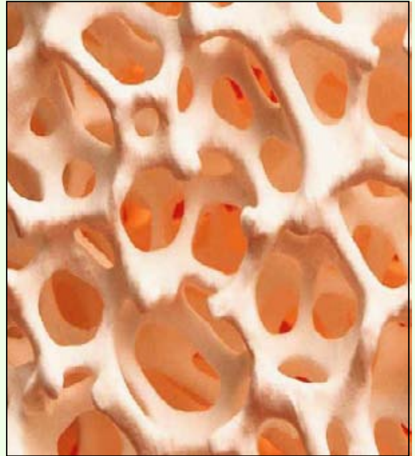
Reticulated ceramic foam for depth filtration
